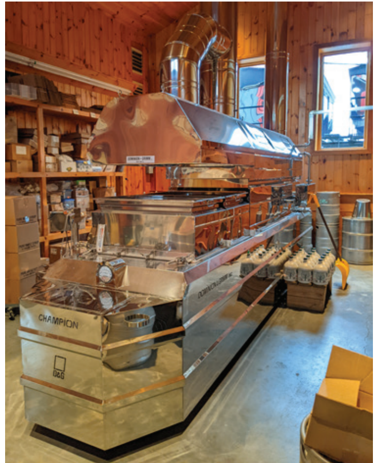
Continuous-feed evaporator at Morning Star Maple. Concentrated sap is boiled down to 66 percent sugar content to create maple syrup.
