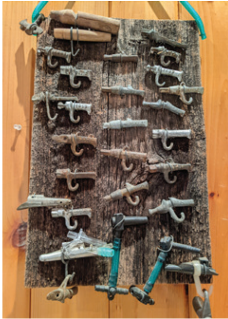
The Keurulainen's collection of spiles used overtime for tapping maple trees. Pails were hung from the hooks before plastic tube pipelines replaced the pails. The oldest metal spile in the collection was patented in 1872.
